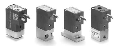
Please note that all Series PD solenoid valves are supplied with direct current (DC). To operate in alternating current (AC), it is necessary to use the connector with bridge rectifier Mod. 125-900.
