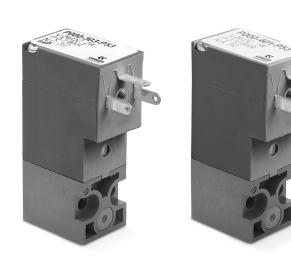
Series P directly operated solenoid valves are available as 3/2-way, either NC or NO. Both versions can be mounted on single sub-bases or manifolds and they are equipped with a monostable manual override. » Can be mounted on a single base (M5 connections) or on manifold (M5 connections or fittings for Ø3 o Ø4 tube).
