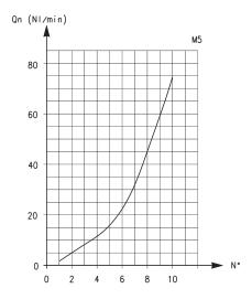
To ensure the right choice of unidirectional flow controller, proceed as follows: calculate the quantity of air in Nl/min (see cylinder Table); determine the stroke time of the cylinder; refer to graph to see which controller is the right type.
