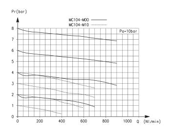
Flow diagram for model: MC104-M00 Pa = Inlet pressure (bar) Pr = Regulated pressure (bar) Q = Flow (Nl/min)
