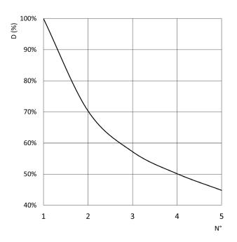
N° = number of valves in manifold configuration D(%) = relative percentage decay of the maximum flow rate Note: the air inlet is only from one side, in case it should be on the right and on the left, only consider the positions as from 1 ÷ 3.
