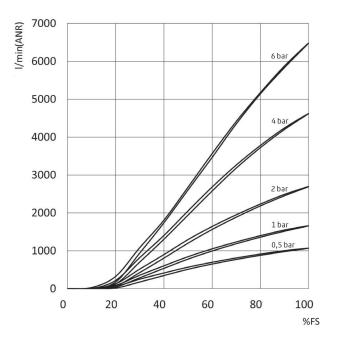
l\min = flow FS = full scale command signal
