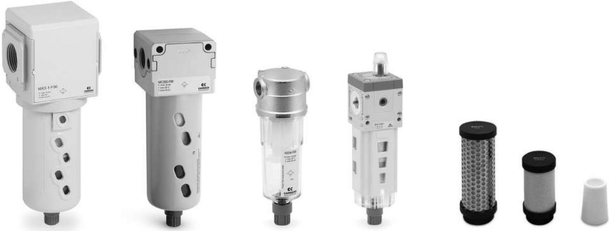
The filters are used to remove impurities in the compressed air, which must then be removed from the pneumatic circuit. The filters can be equipped with different types of drainings of condensate, both automatic and manual. The correct combination and the functioning is reported in the table and in the descriptions on the following pages.
